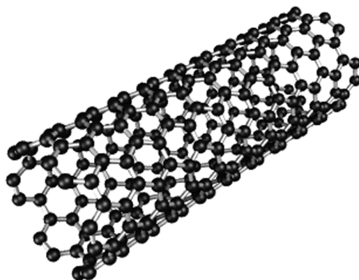
Figure 7. Carbon nanotube structure (image by Eric Weiser under the Creative Commons Attribution-Share Alike 3.0 Unported ( //creativecommons.org/licenses/by-sa/3.0/deed.en ) license.
