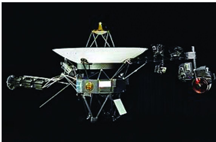
Figure 3. The Voyager spacecraft with its science boom and radioisotope thermoelectric power supply deployed. Courtesy NASA/JPL/Caltech.
